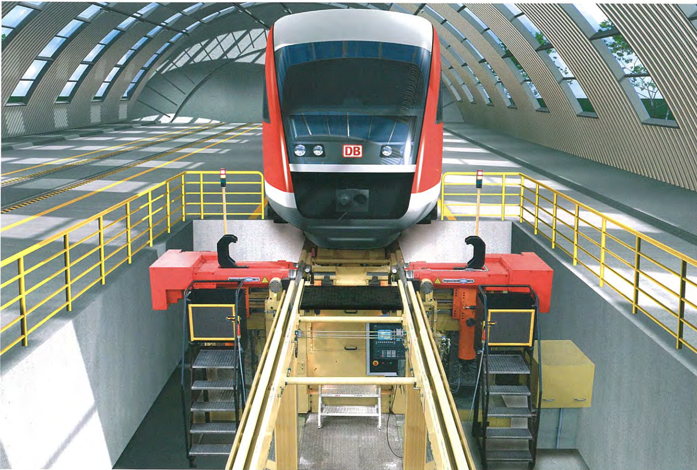
CNC-controlled machine with automatic measuring system
