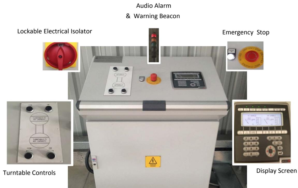
**Figure 2 - Typical Control Console**
