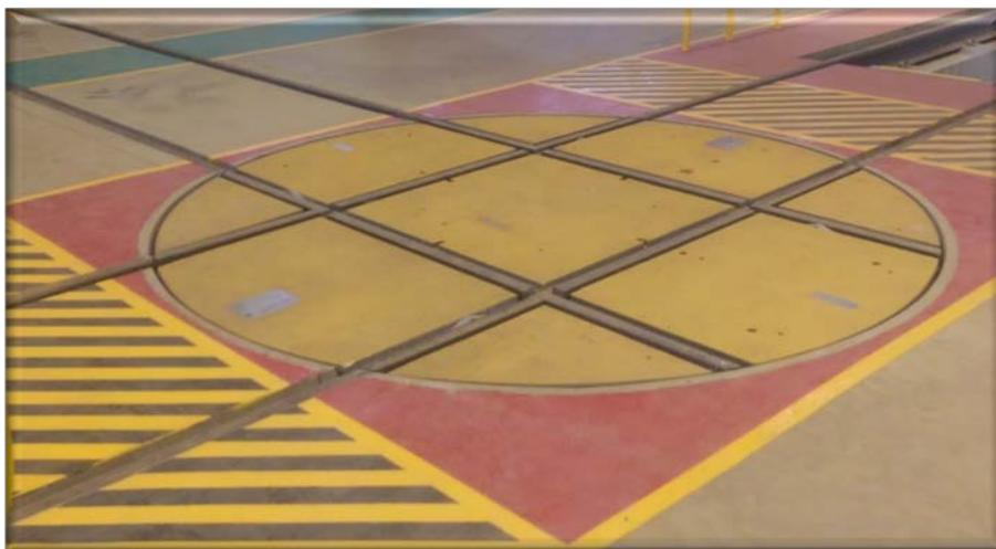
***Figure 1 - Typical 4-Way Turntable***
