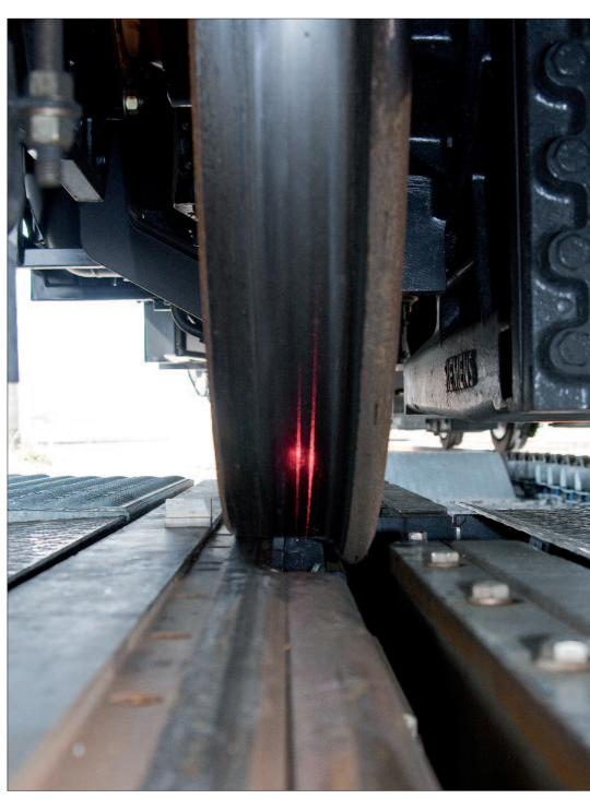
For the inspection of wheelsets on moving trains
